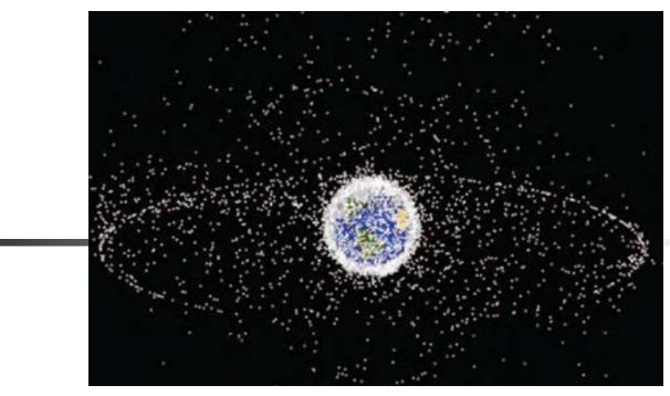
Many artificial satellites have been placed in orbit about the Earth. This diagram shows a plot of all known unclassified satellites and satellite debris larger in size than a baseball. Note the large number of **geosynchronous** satellites that form a visible circle above the Earth's equator.
